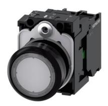
Illuminated pushbutton, 22 mm, round, plastic, clear, pushbutton, flat, momentary contact type, with holder, 1NO, LED module with integrated LED 24 V AC/DC, screw terminal, with laser labeling, symbol number according to, ISO 7000 or IEC 60417
