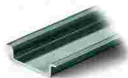
Item no.: 210-113 Steel carrier rail; 35 x 7.5 mm; 1 mm thick; 2 m long; unslotted; according to EN 60715; silver-colored
