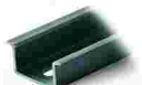
Item no.: 210-197 Steel carrier rail; 35 x 15 mm; 1.5 mm thick; 2 m long; slotted; similar to EN 60715; silver-colored
