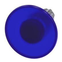
Illuminated mushroom pushbutton, 22 mm, round, metal, shiny, blue, 60 mm, latching, pull-to-unlatch mechanism, with laser labeling, upper case  $\,$
