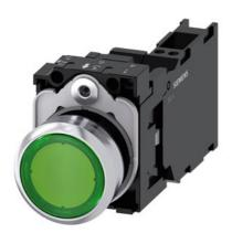
Illuminated pushbutton, 22 mm, round, metal, shiny, green, pushbutton, flat, momentary contact type, with holder, 1 NO+1 NC, LED module with integrated LED 110 V AC, spring-type terminal, with laser labeling, upper case
