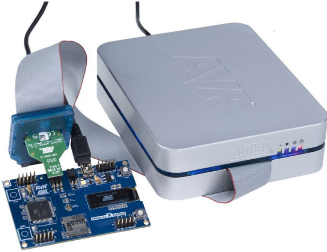
Figure 3-2. Connecting Atmel AVR ONE! to an Atmel XMEGA-C3 Xplained Board
