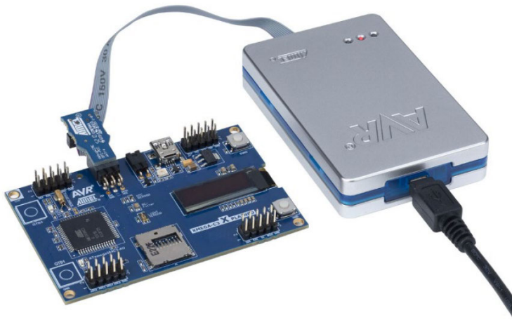
Figure 3-1. The 100mil PDI Adapter must be used to Connect to the Kit
