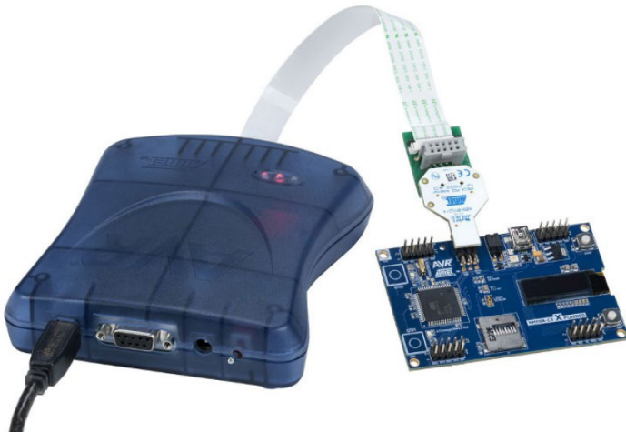
Figure 3-3. Connecting AVR JTAGICE mkII to an XMEGA-C3 Xplained Board
