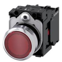
Illuminated pushbutton, 22 mm, round, metal, shiny, red, pushbutton, flat, momentary contact type, with holder, 1NC, LED module with integrated LED 110 V AC, screw terminal, with laser labeling, upper case
