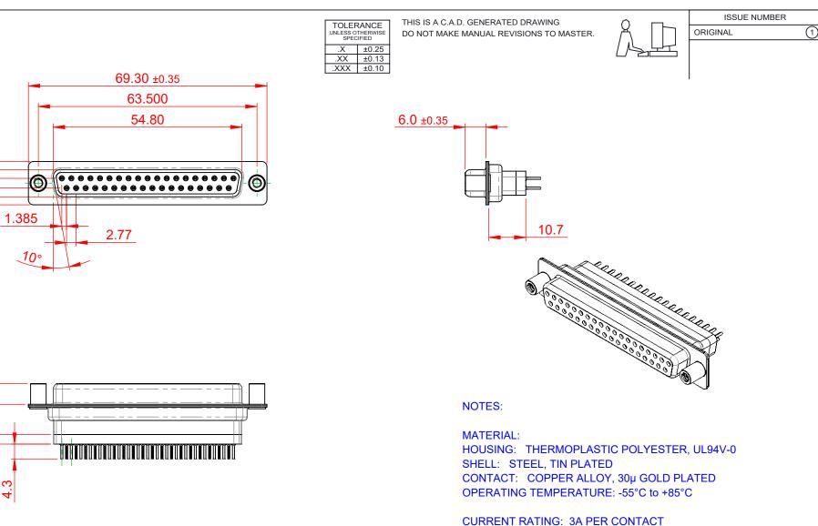
CURRENT RATING: 3A PER CONTACT CONTACT RESISTANCE: 25mΩ MAX. INSULATOR RESISTANCE: 5000MΩ min. DIELECTRIC WITHSTANDING VOLTAGE: 1000V AC rms
