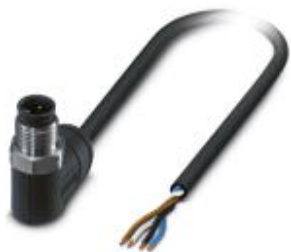
Sensor/actuator cable, 4-position, PE-X halogen-free, black-gray RAL 7021, Plug angled M12, A-coded, on free cable end, cable length: 2 m, for outdoor applications, with high-grade steel knurl
