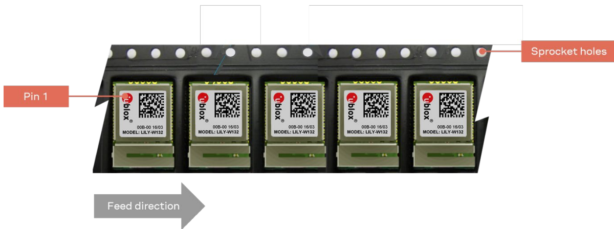
Figure 7: Orientation of LILY-W132 modules on tape
