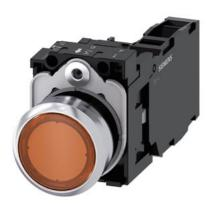
Illuminated pushbutton, 22 mm, round, metal, shiny, amber, pushbutton, flat, momentary contact type, with holder, 1 NO+1 NC, LED module with integrated LED 230 V AC, screw terminal, with laser labeling, upper case and lower case, always upper case at beginning of line
