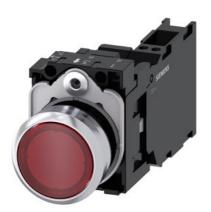
Illuminated pushbutton, 22 mm, round, metal, shiny, red, pushbutton, flat, momentary contact type, with holder, 1 NO+1 NC, LED module with integrated LED 110 V AC, spring-type terminal, with laser labeling, upper case
