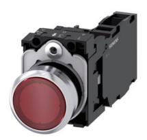
Illuminated pushbutton, 22 mm, round, metal, shiny, red, pushbutton, flat, momentary contact type, with holder, 1 NO+1 NC, LED module with integrated LED 24 V AC/DC, screw terminal, with laser labeling, symbol number according to, ISO 7000 or IEC 60417
