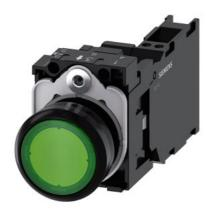
Illuminated pushbutton, 22 mm, round, plastic, green, pushbutton, flat, momentary contact type, with holder, 1 NO+1 NC, LED module with integrated LED 24 V AC/DC, spring-type terminal, with laser labeling, upper case
