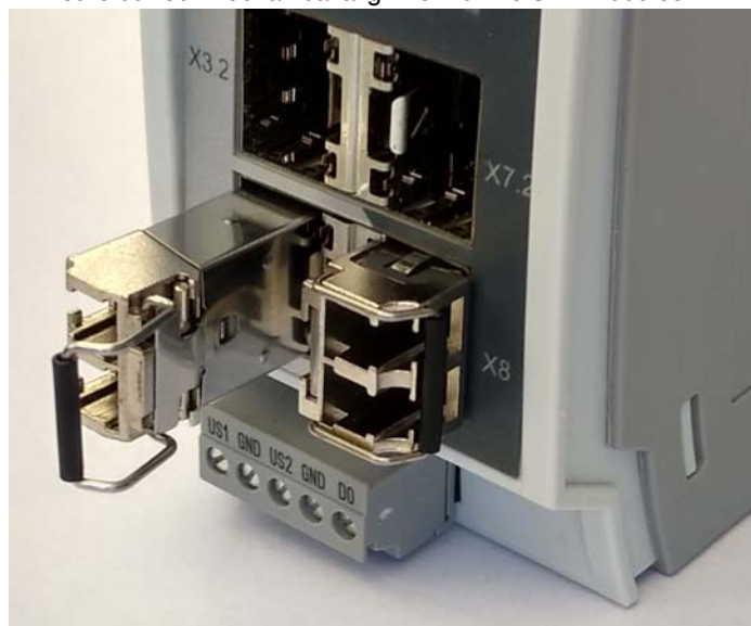
Figure 2-7 Inserting the SFP modules (example)
