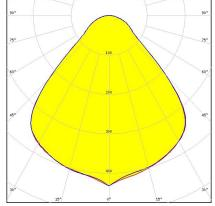
**Dimensions: 35.0 mm x 35.0 mm Height: 15.80 mm** ~90° extra wide beam optimized for LUXEON M/MX. Assembly with holder and installation tape.
