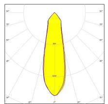
Dimensions: 35.0 mm x 35.0 mm Height: 15.80 mm ~35° wide beam optimized for LUXEON M/MX. Assembly with holder and installation tape.
