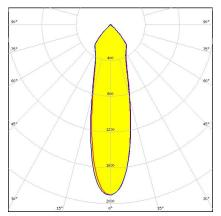
Dimensions: 35.0 mm x 35.0 mm Height: 15.60 mm ~35° wide beam. Assembly with installation tape.
