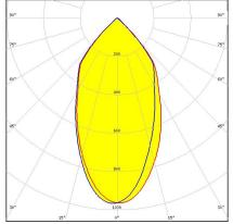
Dimensions: 35.0 mm x 35.0 mm Height: 15.80 mm ~70° very wide beam. Assembly with installation tape.
