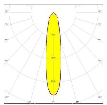
Dimensions: 35.0 mm x 35.0 mm Height: 15.60 mm ~25° medium beam. Assembly with installation tape.
