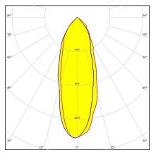
Dimensions: 35.0 mm x 35.0 mm Height: 15.80 mm ~35° wide beam optimized for CREE MT-G. Assembly with holder and installation tape.
