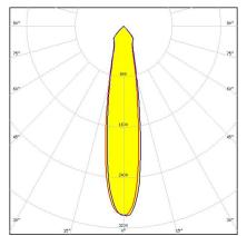
**Dimensions: 35.0 mm x 35.0 mm Height: 15.80 mm** ~25° medium beam optimized for LUXEON M/MX. Assembly with holder and installation tape.
