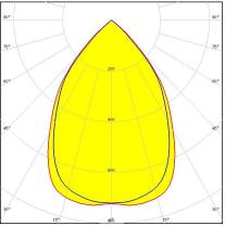
Dimensions: 35.0 mm x 35.0 mm Height: 15.80 mm ~70° wide beam optimized for CREE MT-G. Assembly with holder and
