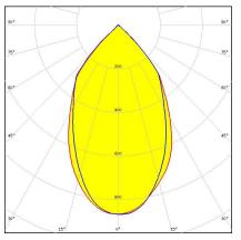
**Dimensions: 35.0 mm x 35.0 mm Height: 15.80 mm** ~70° very wide beam optimized for LUXEON M/MX. Assembly with holder and installation tape.
