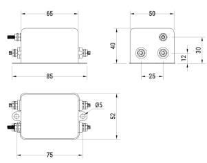
Series FLLE2-Q Style **Chassis Mount** Description Single Phase, Chassis Mount Filters Single Phase Features Phase Single-phase RoHS Yes Qualifications IEC/EN 60939, UL, CSA Threaded Studs M4 **Terminal Type**
