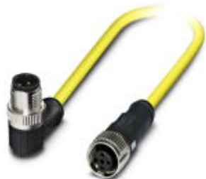
Sensor/actuator cable, 3-position, PVC, yellow, Plug angled M12 SPEEDCON, A-coded, on Socket straight M12 SPEEDCON, A-coded, cable length: 1.5 m
