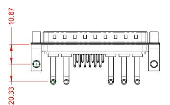
OPERATING TEMPERATURE: $-55^{\circ}C \sim 125^{\circ}C$ POWER/CO-AX CONTACT RATING:20A (CURRENT)(IF PRESENT)SIGNAL CONTACT CURRENT RATING:5A PER CONTACTSIGNAL CONTACT RESISTANCE:10m $\Omega$  MAX.INSULATOR RESISTANCE:5000M $\Omega$  min.DIELECTRIC2000M $\Omega$  min.
