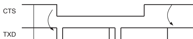
Figure 36-28: Transmitter Behavior when Operating with Hardware Handshaking
