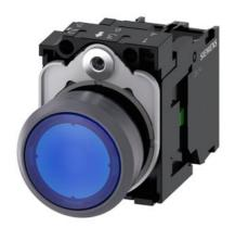
Illuminated pushbutton, 22 mm, round, plastic with metal front ring, blue, pushbutton, flat, momentary contact type, with holder, 1NO, LED module with integrated LED 24 V AC/DC, screw terminal, with laser labeling, upper
