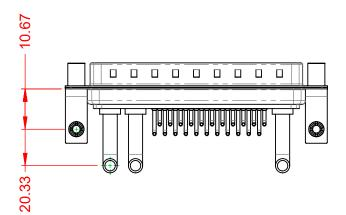
OPERATING TEMPERATURE: $-55^{\circ}C \sim 125^{\circ}C$ POWER/CO-AX CONTACT RATING:40A (CURRENT)(IF PRESENT)SIGNAL CONTACT CURRENT RATING:5A PER CONTACTSIGNAL CONTACT RESISTANCE: $10m\Omega$  MAX.INSULATOR RESISTANCE: $5000M\Omega$  min.DIELECTRICDIELECTRIC
