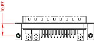
POWER/CO-AX CONTACT RATING: (IF PRESENT) SIGNAL CONTACT CURRENT RATING: 5A PER CONTACT SIGNAL CONTACT RESISTANCE:  $10m\Omega$  MAX. **INSULATOR RESISTANCE:** 5000MΩ min.
