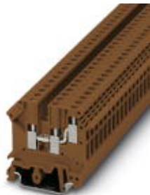
1-level terminal block with double connection on one side, cross section: 0.2 - 4 mm 2 , AWG: 24 - 12, width: 6.2 mm, color: Brown
