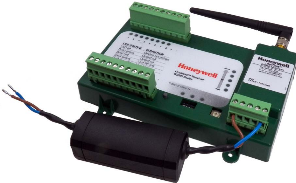
Figure 2. Limitless™ WDRR Din-Rail Receiver with WDRRPWRASM connected
