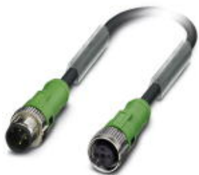
Sensor/actuator cable, 3-position, Variable cable type, Plug straight M12 SPEEDCON, A-coded, on Socket straight M12 SPEEDCON, A-coded, cable length: Free input (0.2 ... 40.0 m)
