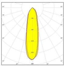
Dimensions: 32.4 mm x 32.4 mm Height: 14.75 mm ~25° medium beam
