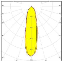
Dimensions: 35.0 mm x 35.0 mm Height: 15.80 mm ~25° medium beam optimized for CREE MT-G. Assembly with holder and installation tape.
