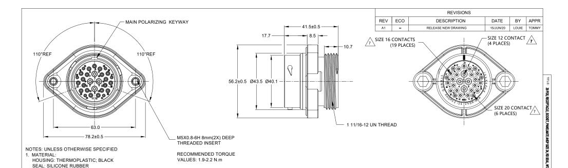
2. MODIFICATIONS: WIDE THREAD ADAPTER (WTA); REDUCED DIA. WIRE SEAL; SEALED PANEL MOUNT
