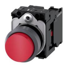
Pushbutton, 22 mm, round, plastic with metal front ring, red, pushbutton, raised, momentary contact type, with holder, 1 NC, screw terminal, with laser labeling, upper case
