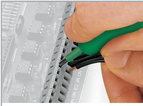
Inserting a conductor via 3.5 mm screwdriver.
