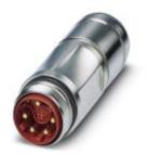
Coupling connector, straight long, shielded: yes, for standard and SPEEDCON interlock, M40, No. of pos.: 8+4+PE, type of contact: Pin, Crimp connection, cable diameter range: 9 mm ... 14 mm
