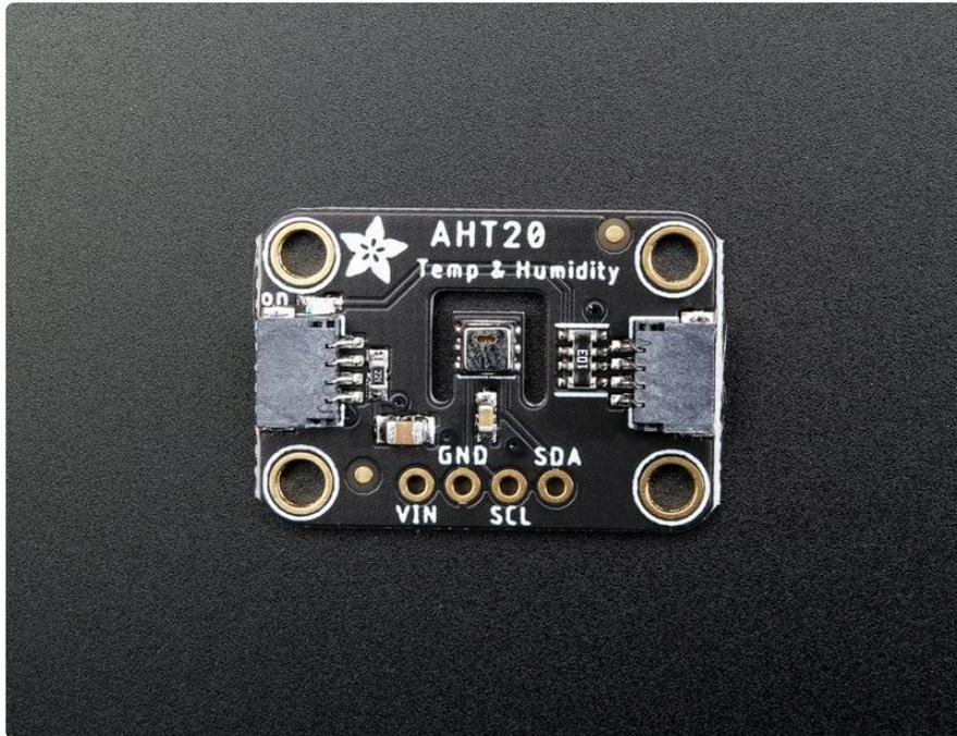
The AHT20 is a nice but inexpensive temperature and humidity sensor [from the same folks that brought us the DHT22 \(\)](#). You can take sensor readings as often as you like, and it uses standard I2C so its super easy to use with any Arduino or Linux/Raspberry Pi board.
