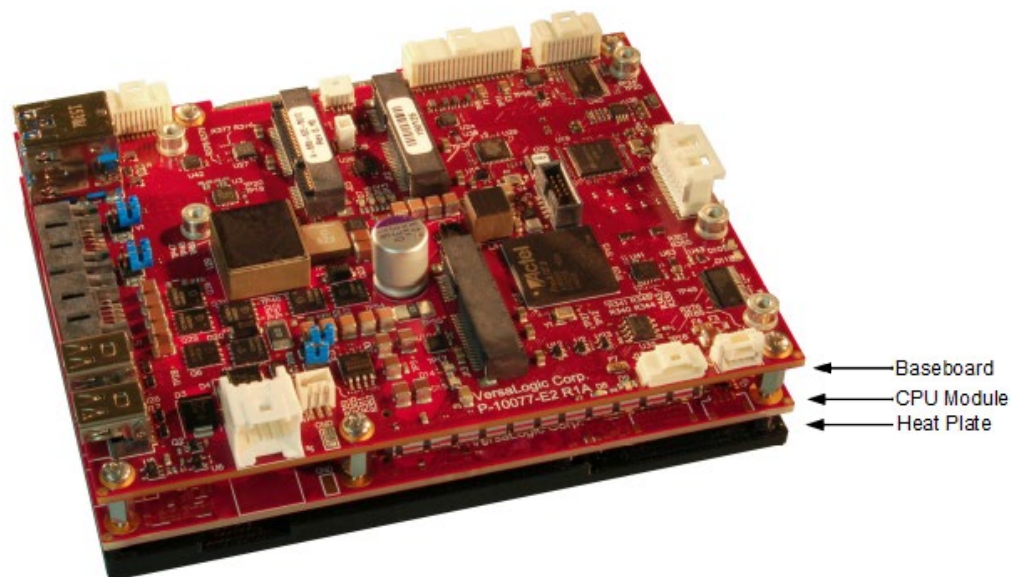
Figure 35. Hardware Assembly with Heat Plate Down
