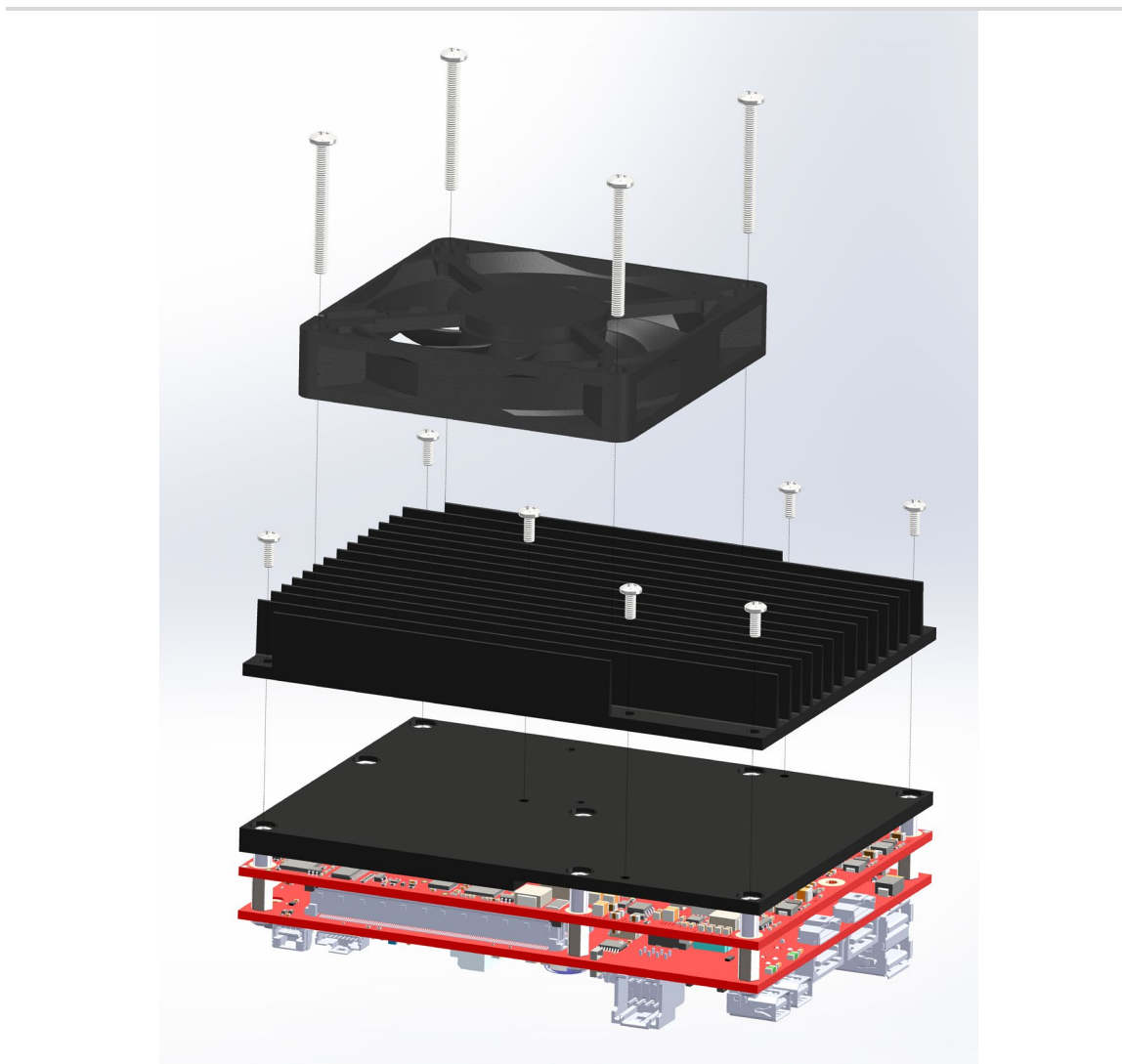
Figure 37. Installing the Heat Sink Fan
