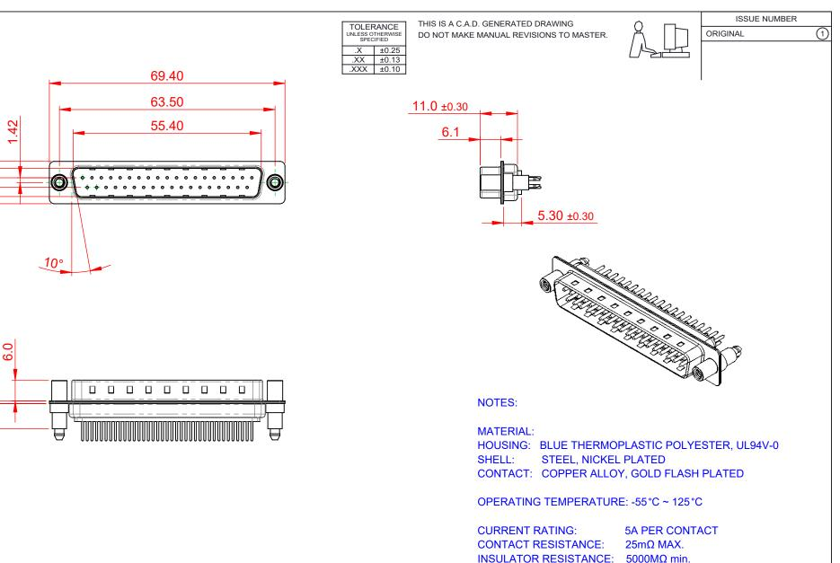
DIELECTRIC WITHSTANDING VOLTAGE: 1000V AC rms
