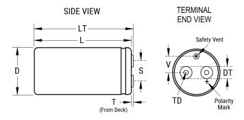
General Information Series ALS40 Dielectric Aluminum Electrolytic Description Screw Terminal, Aluminum Electrolytic RoHS AEC-Q200 No Halogen Free No Component 900 g Weight Dimensions D And L Include Sleeving. MS (MxH) = Notes M12x16. Mounting Clamp (Sold Separately): V90N Shelf Life 156 Weeks
