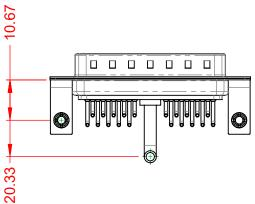
30A (CURRENT) POWER/CO-AX CONTACT RATING: (IF PRESENT) SIGNAL CONTACT CURRENT RATING: 5A PER CONTACT SIGNAL CONTACT RESISTANCE:  $10m\Omega$  MAX.
