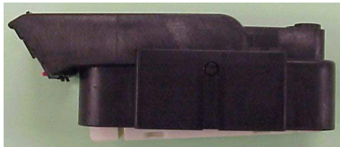
TPA partially seated
