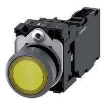
Illuminated pushbutton, 22 mm, round, plastic with metal front ring, yellow, pushbutton, flat, momentary contact type, with holder, 1 NO+1 NC, LED module with integrated LED 24 V AC/DC, screw terminal, with laser labeling, lower case
