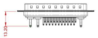
POWER/CO-AX CONTACT RATING:10A (CURRENT)(IF PRESENT)SIGNAL CONTACT CURRENT RATING:5A PER CONTACTSIGNAL CONTACT RESISTANCE: $10m\Omega$  MAX.INSULATOR RESISTANCE:5000MΩ min.DIELECTRICDIELECTRIC
