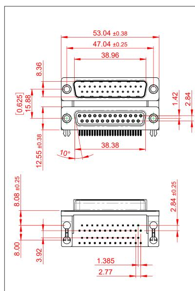
THIS IS A C.A.D. GENERATED DRAWING TOLERANCE UNLESS OTHERWISE SPECIFIED DO NOT MAKE MANUAL REVISIONS TO MASTER. .X ±0.25
