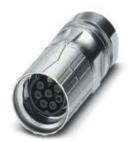
Cable connector, straight, SPEEDCON locking, M17, number of positions: 7+PE, type of contact: Socket, Crimp connection, shielded: yes, cable diameter range: 10 mm ... 12.5 mm
