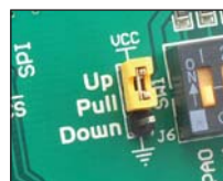
Figure 13-3: J2 in pull-up position
