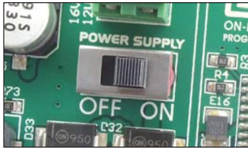
Figure 1-3: Power supply on/off switch
