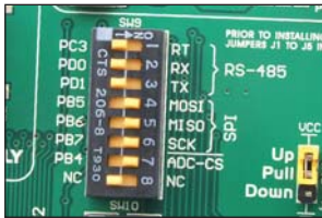
Figure 7-3: DIP switch SW9
