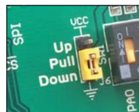
Figure 13-2: J2 in pull-down position
