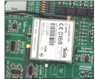
Figure 9-3: Telit's GM862 module
