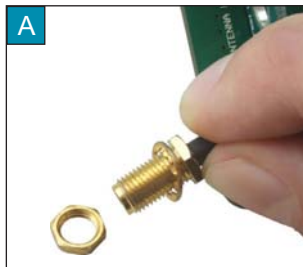
Figure 9-4: Screwing cable into antenna holder
