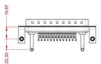
20A (CURRENT) POWER/CO-AX CONTACT RATING: (IF PRESENT) SIGNAL CONTACT CURRENT RATING: 5A PER CONTACT SIGNAL CONTACT RESISTANCE:  $10m\Omega$  MAX. **INSULATOR RESISTANCE:** 5000MΩ min. DIELECTRIC
