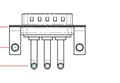
30A (CURRENT) POWER/CO-AX CONTACT RATING: (IF PRESENT) SIGNAL CONTACT CURRENT RATING: 5A PER CONTACT SIGNAL CONTACT RESISTANCE:  $10m\Omega$  MAX.
