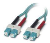
Assembled FO cable, zip cord cable, multi-mode fiberglass 50/125  $\mu$ m, OM3, plug: SC duplex/SC duplex, degree of protection: IP20, for installation in cable ducts or control cabinets, length: 2 m
