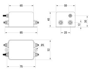
**General Information** Series FLLE2-P Style **Chassis Mount** Description Single Phase, Chassis Mount Filters Single Phase Features Phase Single-phase RoHS Yes Qualifications IEC/EN 60939, UL, CSA Threaded Studs M4 **Terminal Type**
