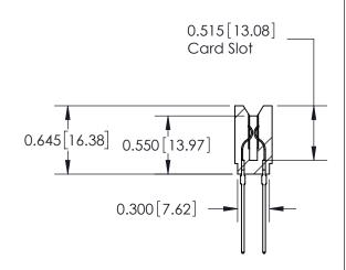
737 Series Ultra-Mate Card Edge Connector - Press Fit
