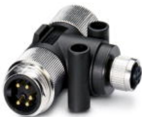
Bus system T-connector, DeviceNet™, 5-position, unshielded, Plug straight 7/8"-16UNF, on Socket straight M12, A-coded and Plug straight 7/8"-16UNF, Parallel distributor
