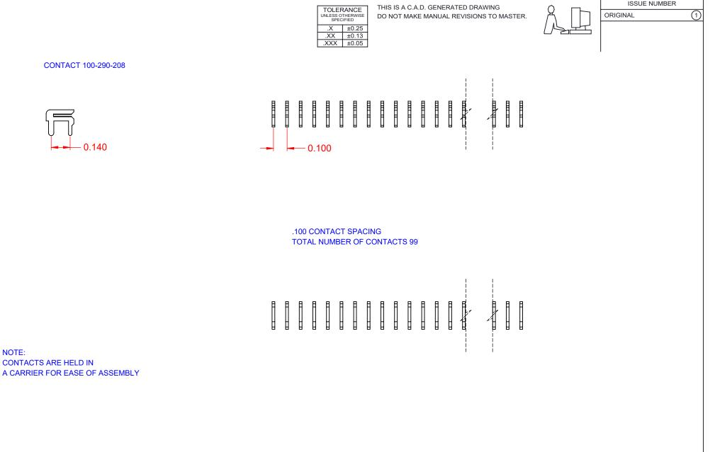
ACAD REFERENCE NO .: 105 Assembly **105 SERIES - VERTICAL CONTACT PATTERN** DRAWN: C.B DATE: April 8, 2020 CHECKED: DATE: THESE DRAWINGS AND SPECIFICATIONS SCALE: 2:1 SHEET 1 OF 1 EDAC INC ARE THE PROPERTY OF EDAC INC..AND TORONTO, ONTARIO SHALL NOT BE REPRODUCED, OR COPIED ISSUE DRAWING NUMBER: 105 Assembly OR USED AS THE BASIS FOR THE CANADA MANUFACTURE OR SALE OF APPARATUS 1 YOUR CONNECTION TO QUALITY & SERVICE PART NUMBER: 105-099-208-100 WITHOUT WRITTEN PERMISSION.
