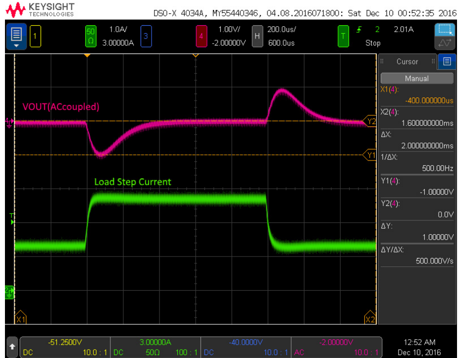
Figure 6. Load Transient Response (Conditions: V_{PORT} = 41.2V , Load Step: 1.35A to 2.7A to 1.35A)
