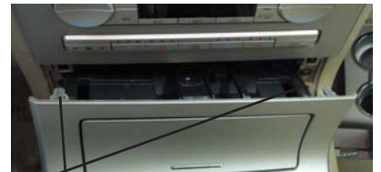
(2)Clips to Remove Ash Tray
