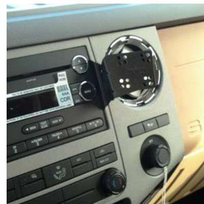
Final Installation Picture of Super Duty 2013 Without NAV
